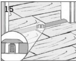
An expansion gap T-strip is required when length of planks measures 102cm max and when width of planks measures 63cm max. Transition strips should be placed in all doorways directly under the door when the door is closed.
