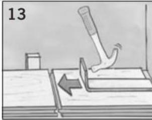
Fit the last panel in the row using a pull bar.
