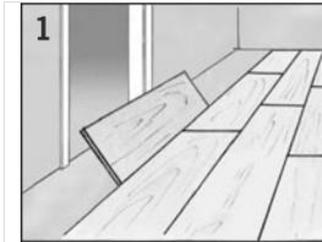
Some long edge joints cannot be installed using a 20° angle.
