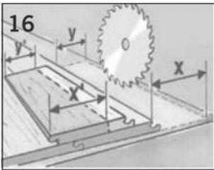
Cut the row along the wall to account for the unevenness of the wall while leaving 1cm expansion room (6cm minimum plank width).
